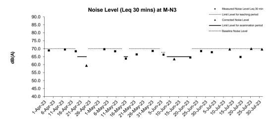
Free field noise levels were adjusted with a correlation of +3 dB(A).
